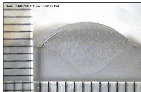
**Fig. 1: The bead geometry with measurement scale**
